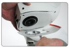
3. Insert the dovetail of the module into the stand. (Analyzer/Bertrand Lens Module shown).
